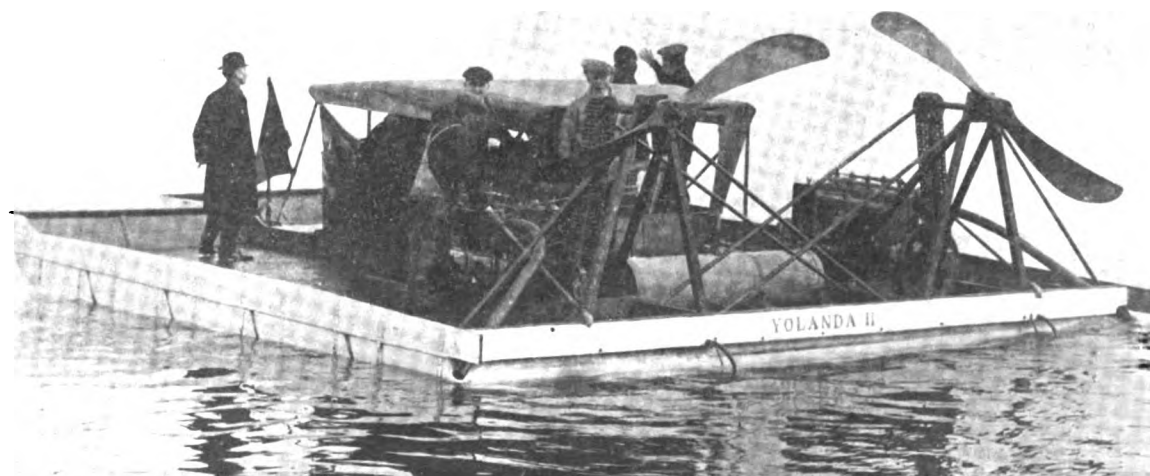
Stern View Showing Chain Drive to Air Propellers
